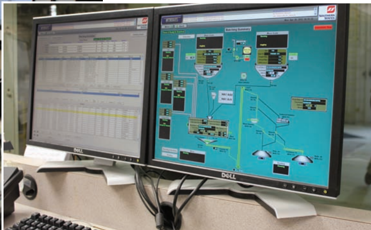
Marty Wilson, batch mix operator, mans the formula feed manufacturing process using ICSI's batch mixing operation controller on the right screen and the the batch scheduling/queuing controller on the left.
