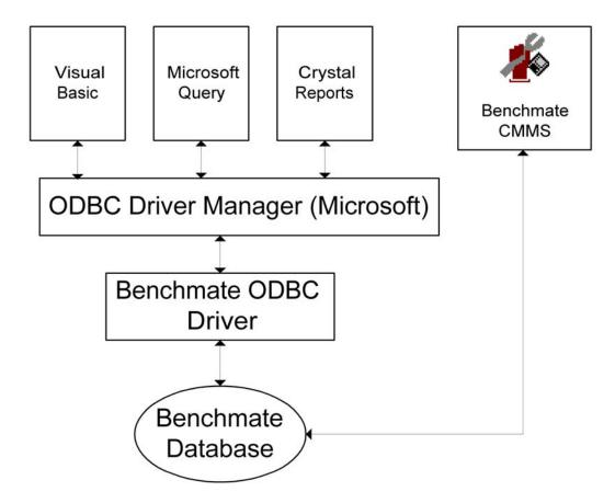
The Benchmate ODBC driver, consisting of components by Faircom Corporation and Benchmate Systems, Inc. translates standard ODBC function calls from the application program (e.g.: Crystal Reports) into calls the Benchmate database can process, and returns data to the application. Any Microsoft Windows tool or application that supports the ODBC call library can use the Benchmate CMMS database.
